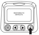
Custom Setup- To perform a custom setup of the 1-Up Display, use the arrow buttons to scroll to and highlight "Custom Setup" on the display.
